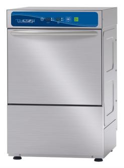
The STEEL line models are equipped with an automatic water softener that offers the possibility to break-down the formation of limestone with extreme efficiency. In fact, the water softener is completely autonomous and automatically controls its regeneration intervals according to the hardness of the inlet water; all you have to do is fill the salt tank whenever the message "lack of salt" appears on the display. The resins are regenerated during wash cycles, so no machine downtime is required.
